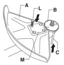
Screw on the trimmer head (H) in the opposite direction to the direction of rotation.
